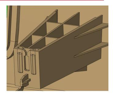
Remember to reduce the clip housing to allow the slide construction. Report already sent. Try to implement a centering boss (Y) without increasing the depth.
