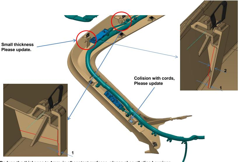
Reduce the thickness to 1mm. in all contact surfaces, please chec all clips housings
